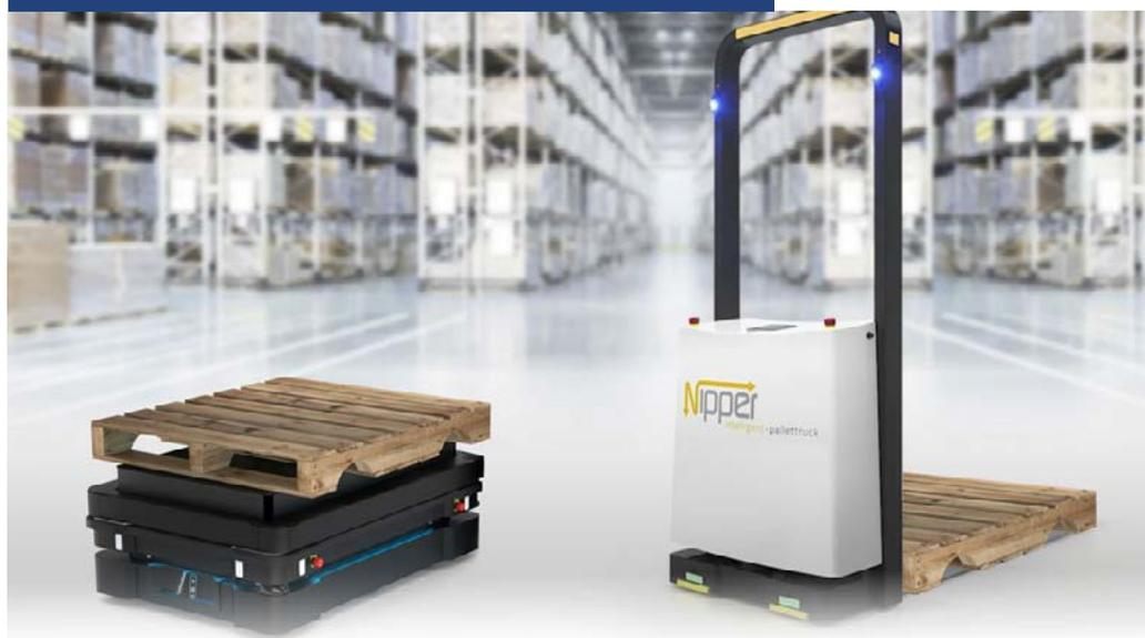
Autonomous Mobile Robots (AMR) are self-driving collaborative vehicles that navigate around people and objects without the need of a track. The flexibility of AMRs is endless. Interchangeable top modules allow for materials of different shapes and sizes. By using AMRs for automated pallet transport, employees' time can be repurposed from point-to-point transportation to focus on more value-added operations.
