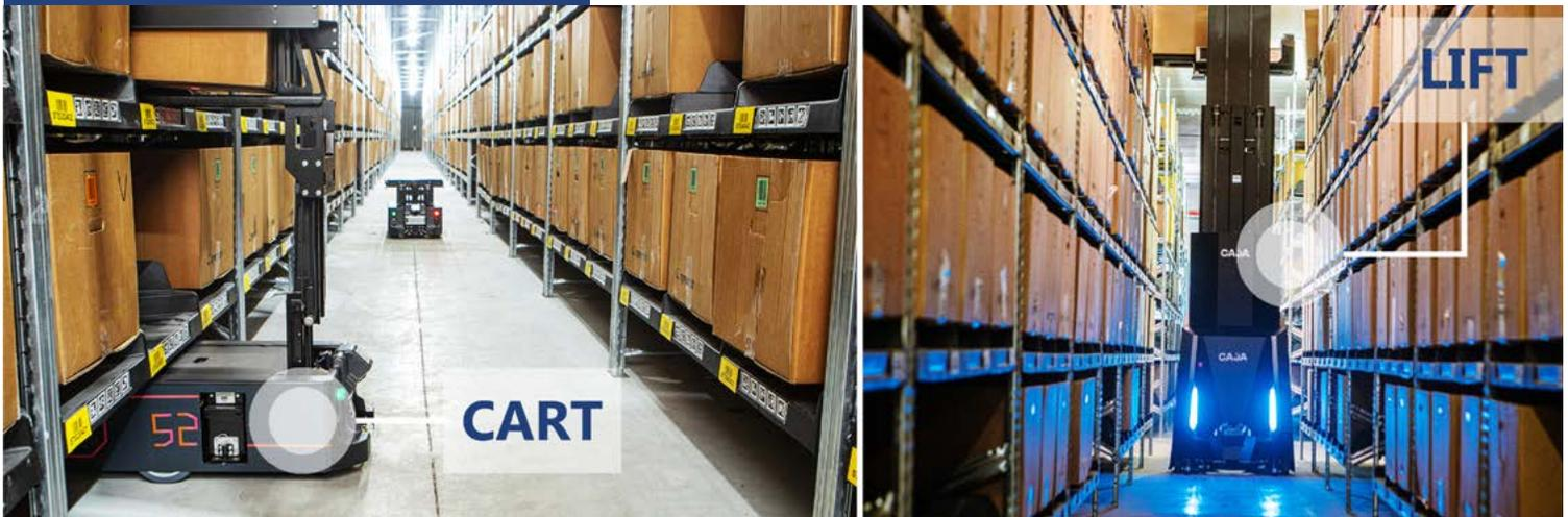
Caja Robotics' two types of specialized robots work synergistically to optimize the goods-to-person system. As the Lift robot can reach high and the Cart robot can move fast, each of them is assigned suitable tasks to constantly move bins between workstations and shelves.
