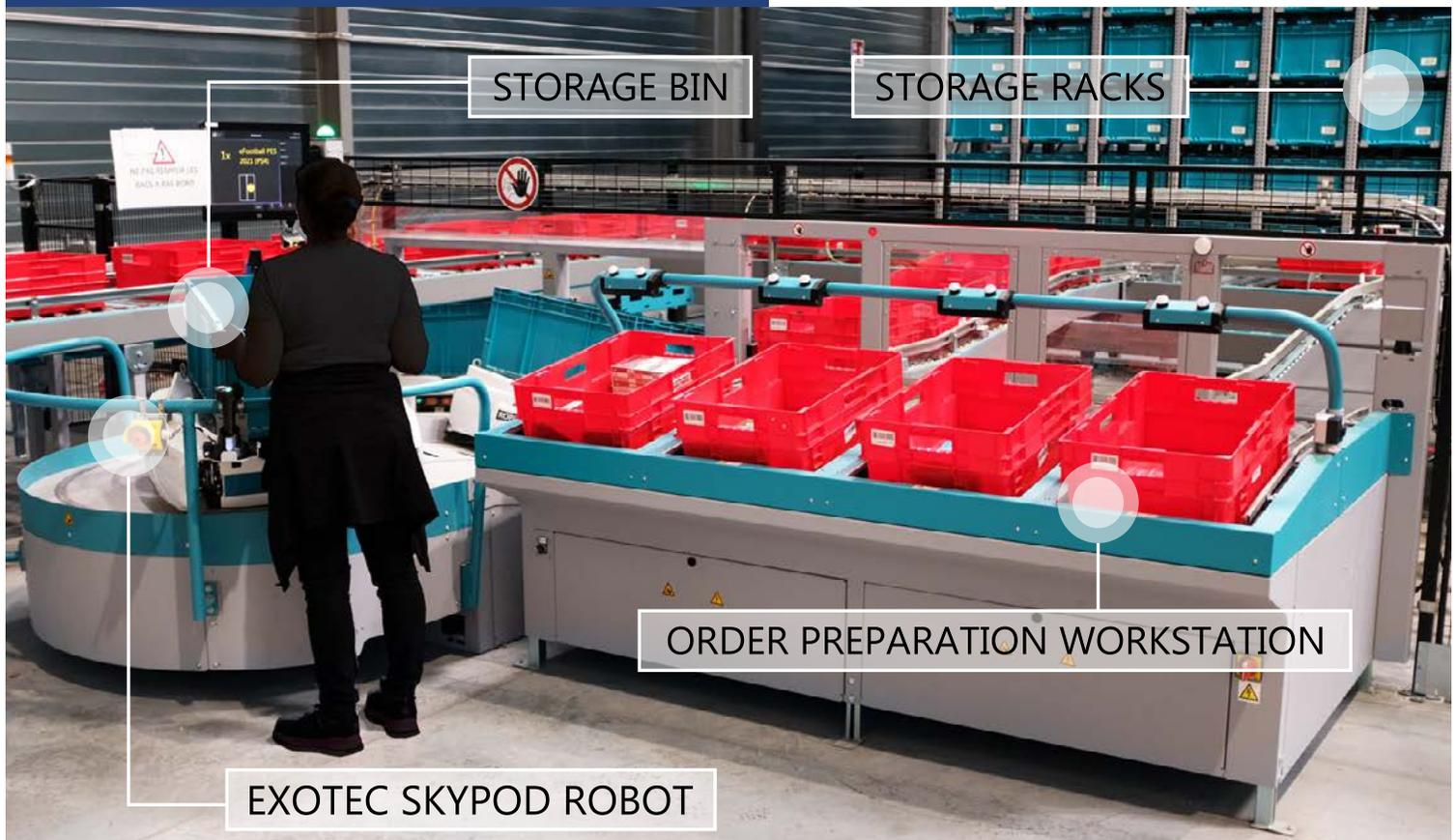
The Exotec Skypod System is an automated storage and order preparation system. The Skypod Robots can climb the multi-level storage racks and move three dimensionally to retrieve the storage bins.
